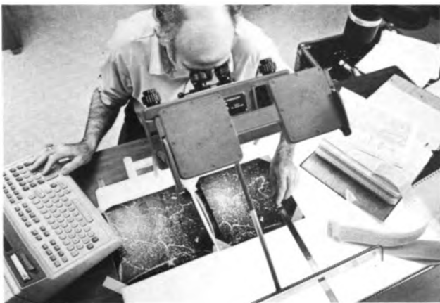
Figure 6-1. — In the PISYS system, an operator views aerial photographs using a scanning stereoscope. Points on the photographs are digitized with a Numonics graphics calculator interfaced to a desk-top minicomputer.
