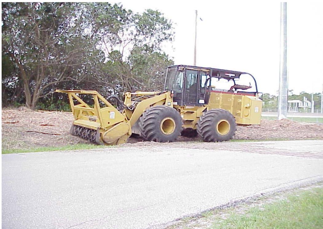
Figure 18. Front end loader in Port St. Lucie fitted with cutting/grinding attachment for removal of Brazilian peppertrees along roadside rights-of-way (Photo credit: J. Dunton).
