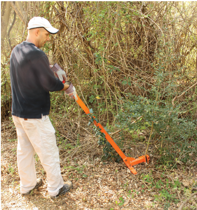
Figure 2. The weed wrench uses leverage to easily lift privet saplings out of the ground.
